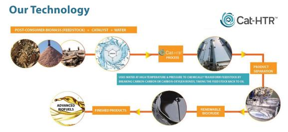
Cat-HTR is world-leading technology that uses heat, pressure and water to break up waste wood biomass and turn it into a low carbon bio oil. As the next-generation of advanced recycling, it takes a process requiring millions of years in nature and drastically shrinks the time – to approximately 20 minutes – to convert woody waste biomass into a renewable and sustainable source of cleaner energy.
