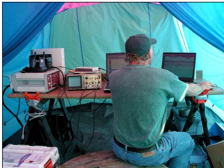
A technician observes hydroacoustic data (left) generated by the system's sound wave producing transducer (right) mounted in the Fraser River near Woodpecker Rapids. 2006 was the second year that Lheidli completed a Treaty Related Measure project to assess the use of this technology for estimating the number sockeye and Chinook migrating through the area.
